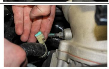
18. Reinstall the cross over pipe clamps (11 mm) and slide them down the pipe. Install the bolt (8mm) located at the center of the pipe, and tighten the clamps.
