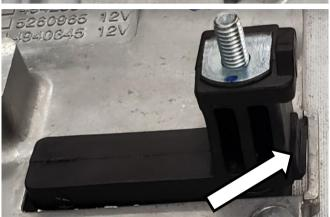
2. To remove the lower busbar, use the included IP25 Torx Plus bit and compact 10mm wrench to remove the bolt and nut in between the heating elements.
