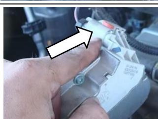
23. Remove the power wire from the grid heater (10 mm).
