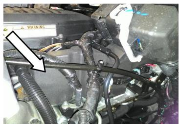
15. Disconnect the high pressure lines from the rail. 2019-2020 models with the CP4 injection pump will have two high pressure lines. The remaining models, including 2021+, will have one high pressure line.
