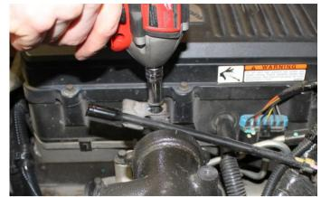
16. **For 2013+ models:** Reinstall the heatshield covering the intake control valve.
