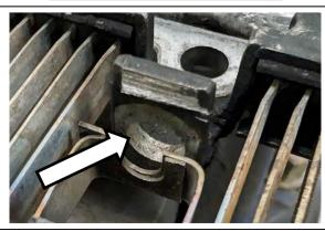
4. For 2007-2012 Models: the grid heaters will require modification before proceeding with installation. These grid heaters have a casting feature that bridges where the heating elements connect to the body of the heater and needs to be cut to be removed.
