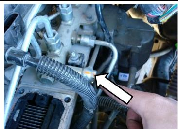
18. For 2019+ Models: Remove the fuel return line (1) by removing the fuel return line banjo bolts (2, 3, 4).
