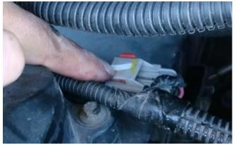
22. Disconnect the EGR servo motor connector.
