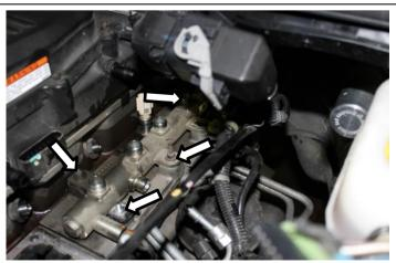
3. Reinstall the six injector lines (19mm). Torque to 30 ft-lbs (40.7 Nm).
