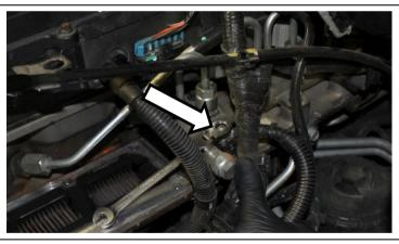
7. Install the heater cable to grid heater stud using the supplied Nyloc nut. Tighten to 9 ft-lbs (12.2 Nm).
