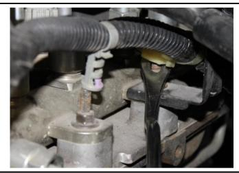
14. For 2013+ Models: Remove the sound deadening foam rubber from around the fuel injection lines to allow access to the fuel lines.
