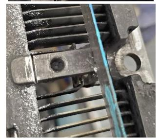
6. Install the nylon insulating washer to the bottom of the grid plate with the washer shoulder pressed firmly into the bolt hole.
