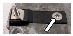
11. Tighten the lower busbar bolt to the heating elements to 7 ft-lbs (9.5 Nm).
