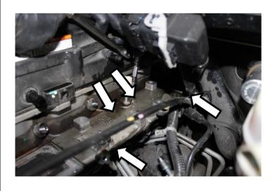
2. Reconnect the fuel rail connector. Then apply some pipe dope to the four OEM fuel rail bolts and install the fuel rail to the intake plate. Torque to 18 ft-lbs (24.4 Nm).
